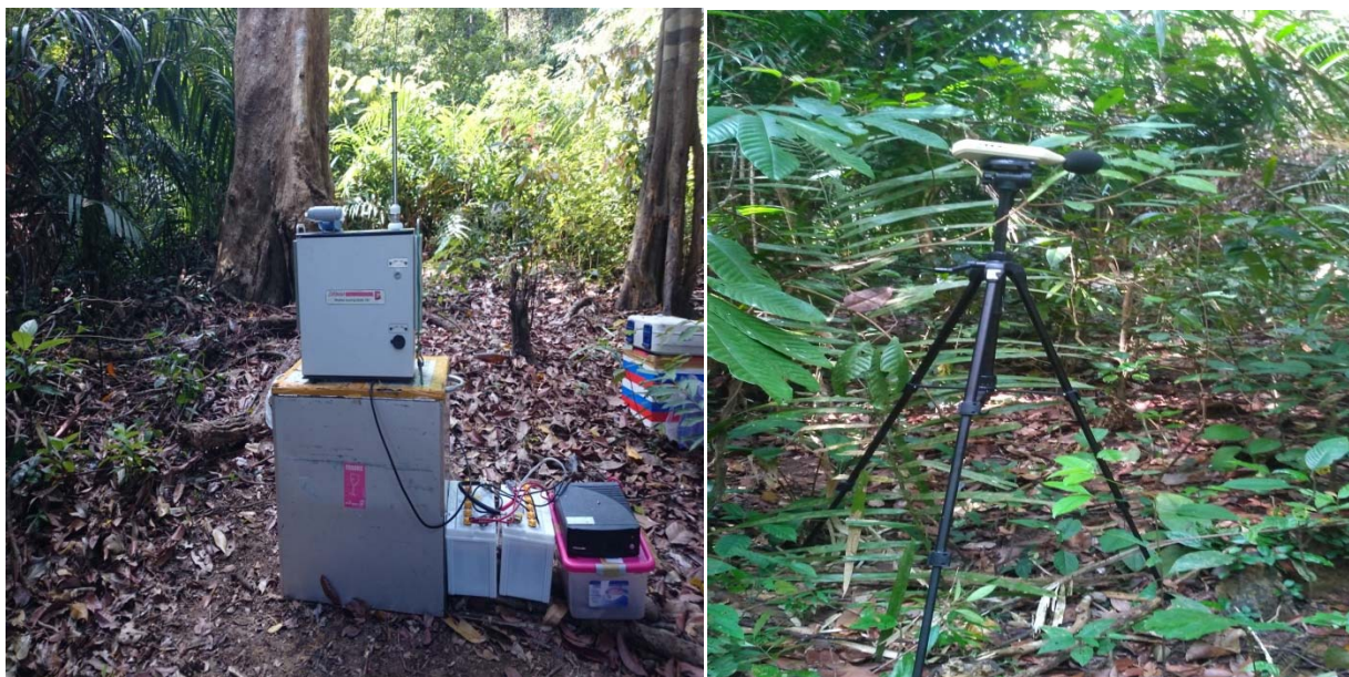
Figure 4.3 Air quality and Noise quality monitoring at Wa Ale island, Air Station- 2, 24 hrs continuous)
